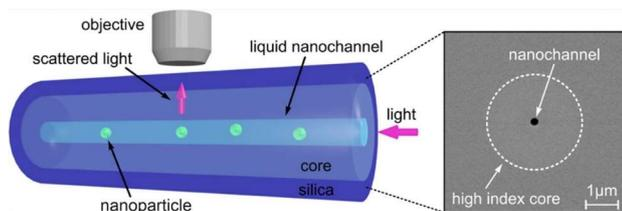
Figure 1: A 633 nm laser is coupled to the fiber, and the light scattered from single-particles is imaged onto a camera through a microscope aligned perpendicularly to the fiber axis.
