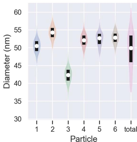
Figure 4: Examples of the uncertainty in size-measurements derived from the scattered intensity of 60nm polystyrene particles.
