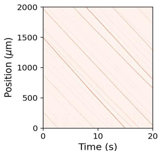
Figure 2: 60 nm polystyrene particles diffusing in a nano-channel, at 200 fps.
