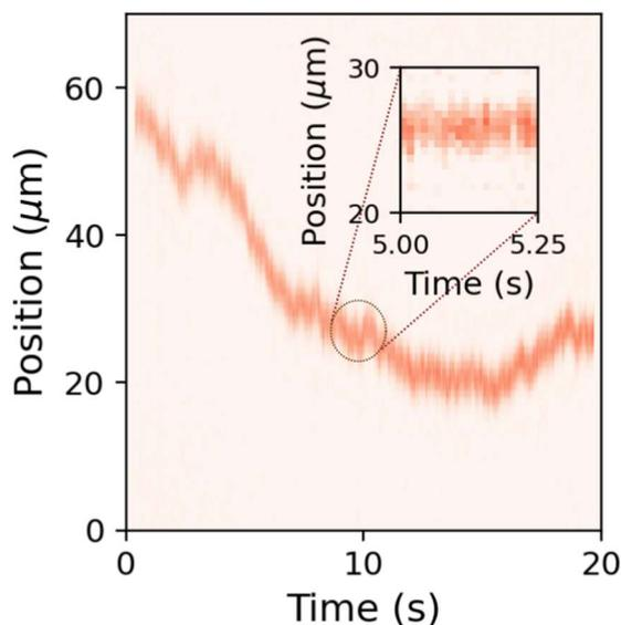
Figure 3: Trace of a 60 nm polystyrene particle after correcting for the fluid drag. The inset shows a detail of the trace where each individual frame and pixel can be recognized.
